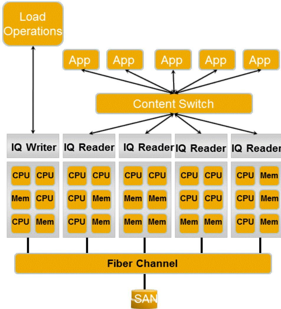
Figure 1 – IQ Multiplex with Content Switch
