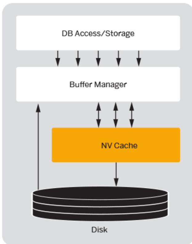
Figure: NV Cache Extension Architecture
